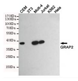
Western blot detection of GRAP2 in GRAP2 positive cell (CEM,Molt-4,Jurkat) and negative cell (3T3,K562,Hela) lysates using GRAP2 mouse mAb (1:1000 diluted).Predicted band size:38KDa.Observed band size:38KDa.
